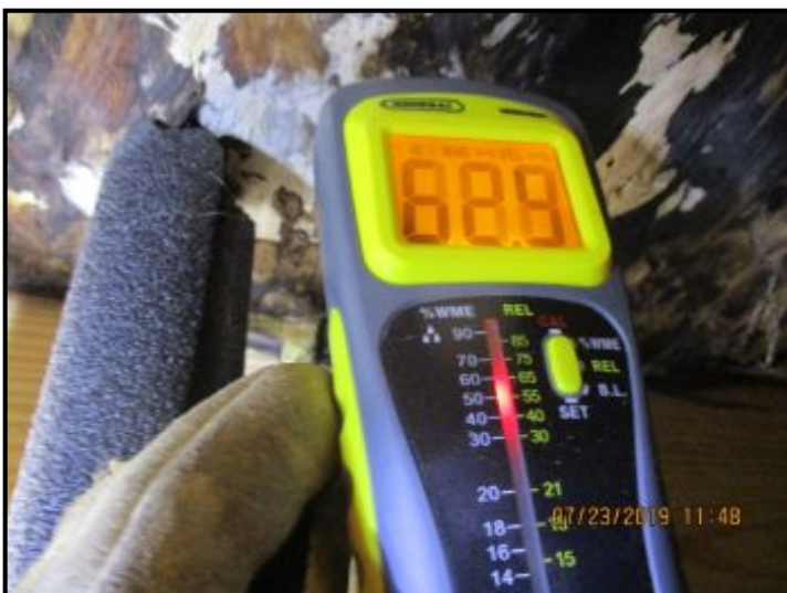
Area under shower drain - 19% moisture content. Area under water heaters - 63% moisture content.
