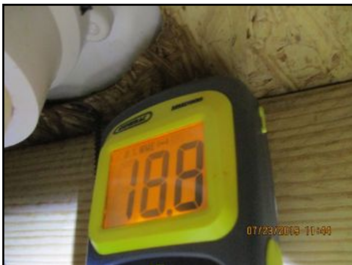
Area under shower drain - 19% moisture content. Area under water heaters - 63% moisture content.
